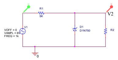
The circuit above is a zener diode voltage regulator. Assume the zener voltage of the diode is 4.7 volts and its forward bias voltage is 0.7 volts.
