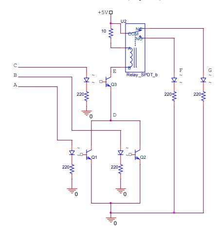
Above is an optical isolation circuit with LED/phototransistor pairs. The inputs may be in a cage whose reference voltage is 5kV higher than the phototransistor and relay circuit, but the "optical isolation" removes the danger of high voltage getting through. The on resistance of the phototransistors is  $20\Omega$  and the resistance of the coil is negligible, although 50mA is needed to turn on the relay.
