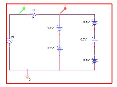
5. (*8pt, 2pt each*) What is the value of current through the resistor R1 when the input voltages are the following: (reminder: Assume Von for each diode is 0.6V)
