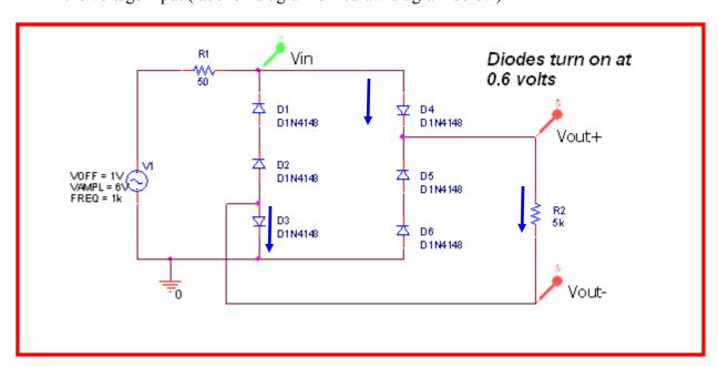
3. (3pt) Draw the current direction through the diodes and resistor, R2, for the negative cycle of the voltage input (label on diagram or redraw diagram below)
