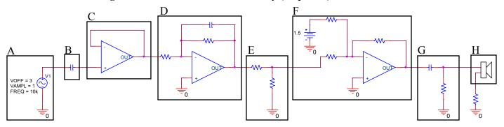
1. (8pt) Identify the function of each of the blocks in the signal conditioning circuit above.
