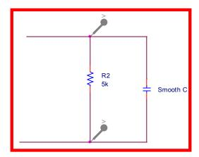
The capacitors store charges from the current due to the voltage across the output. It will then discharge according to its characteristic time. The capacitor can be chosen to have a large time to discharge causing it to smooth the ripple.
