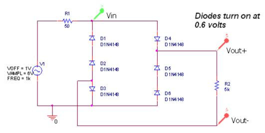
4. (6pt) What will the voltage between Vout+ and Vout- be for the following input voltages:
