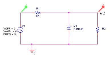
The circuit above is a zener diode voltage regulator. Assume the zener voltage of the diode is 4.7 volts and its forward bias voltage is 0.7 volts.
