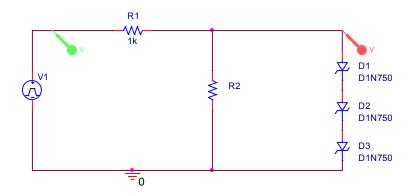
The circuit above is a zener diode voltage regulator. Three Zener diodes are used to regulate the voltage across the load resistor R2 in the circuit below. Three different values of R2 are tried (100 $\Omega$ , 1k $\Omega$ , and 10k $\Omega$ ) Draw the voltage on the output probe above D1. *Calculate your answers.*
