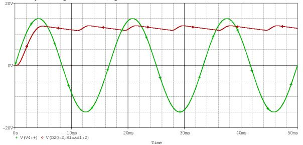
a) (*3pt*) On the plot, show how the voltage across the load would change if Rload is reduced to  $50\Omega$ .
