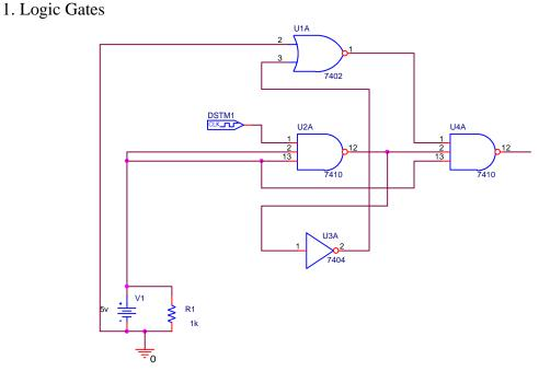
In this circuit, there is a NOR gate (U1), two NAND gates (U2 & U4) and an invertor (U3). Input 2 to the NOR is LO, inputs 2 and 13 to the first NAND are HI, input 1 of the first NAND goes HI and LO (clock), the input to the invertor is the output from the NAND, the output from the invertor is input 3 of the NOR, input 13 of the last NAND is HI, input 2 is the output from the first NAND and input 1 is the output from the NOR.
