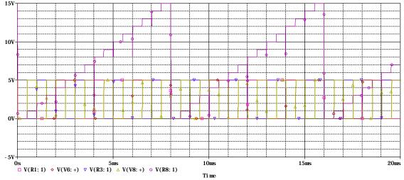
You can see that it does indeed count from 0 to 15 as it should for TTL input levels.
