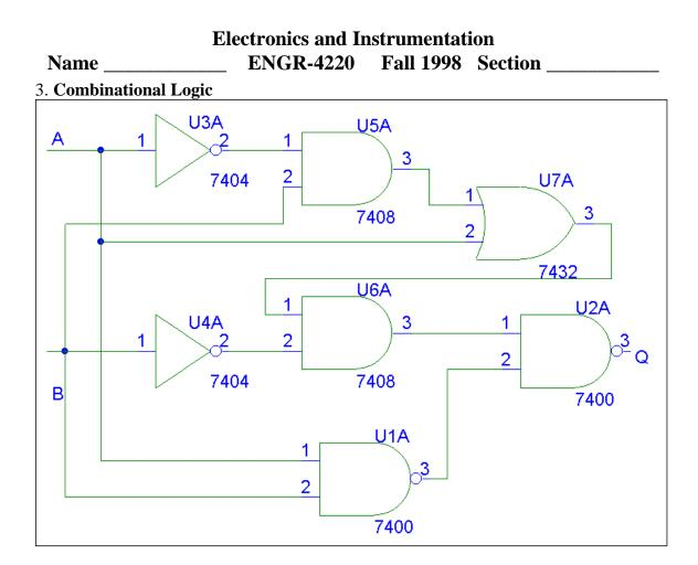
Which of the following truth tables is correct for this circuit?
