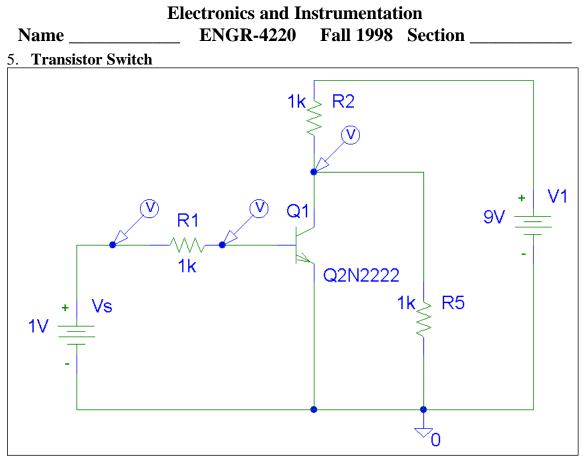
In the circuit above, the voltage source Vs is ramped up from zero to 9 volts and the voltages at the source and two other points are monitored. Which of the following plots goes with this circuit?
