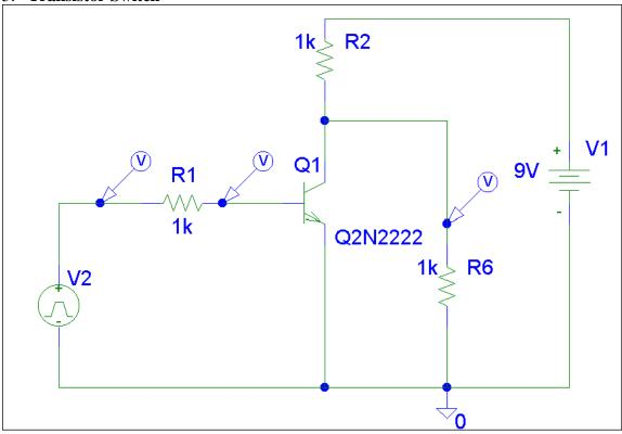
In the circuit above, the voltage source V2 puts out a sequence of pulses and the voltages at the source and two other points are monitored. Which of the following plots goes with this circuit?
