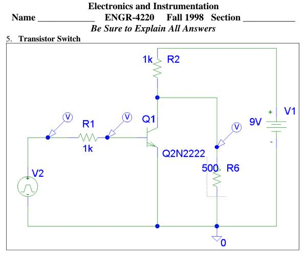
In the circuit above, the voltage source Vs is ramped up from zero to 9 volts and the voltages at the source and two other points are monitored. Which of the following plots goes with this circuit?
