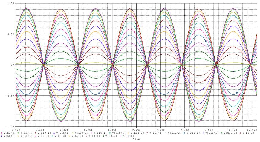
These are the measurements when the frequency is 3.5MHz. Note that the amplitude is not zero at any node. Also note that the signals appear to all be in phase. This is because we are looking at the effects of a standing wave in which the total signal is indeed in phase within each half wavelength. Try the java applet at <a href="http://bessernet.com/Ereflecto/tutorialFrameset.htm">http://bessernet.com/Ereflecto/tutorialFrameset.htm</a> and you will see this effect.
