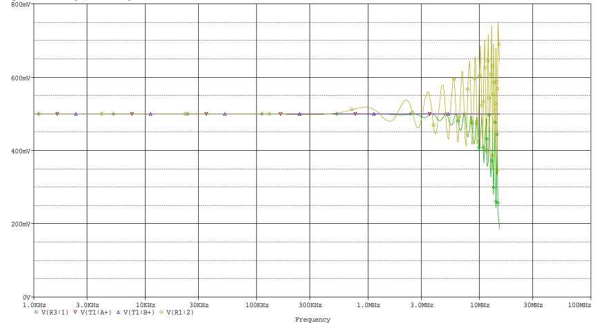
The frequency scan shows that the lumped model is reasonably accurate up to around 1MHz. Compare the input (red and yellow) and output (blue and green) voltages to see this.
