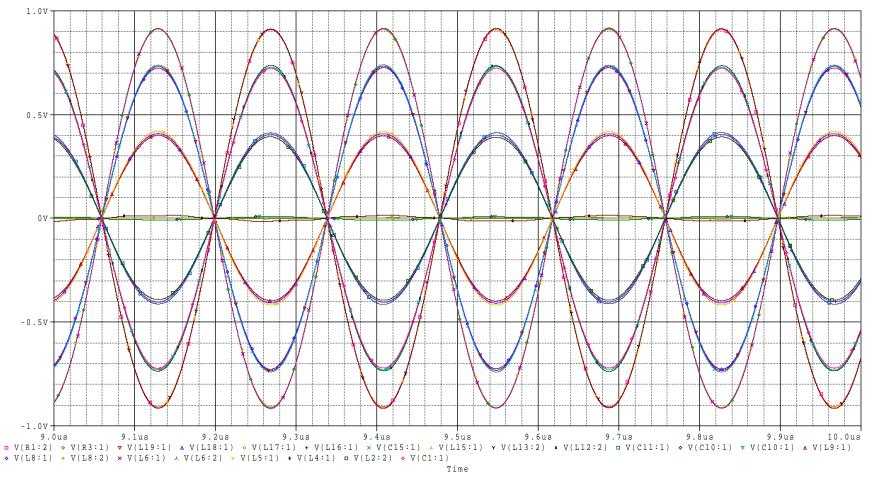
These are the measurements made at all of the nodes when the frequency is 3.58MHz. Note that there are a few nodes where the amplitude is very small. When you do the experiment in JEC 4107, you should see voltages like these. Of course, you can only measure them two at a time with the scope.
