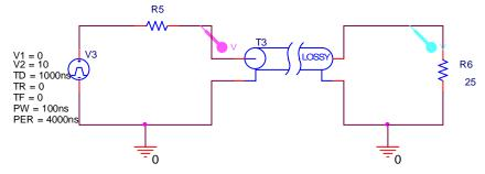
Now run your simulation again, which should simulate both the sinusoidal and pulsed cases simultaneously. You should observe pulses at the input and output ends of the line. It might be helpful to show the sinusoidal and pulsed cases on two separate plots, which PSpice will allow you to do. Now adjust the simulation profile until your plot
