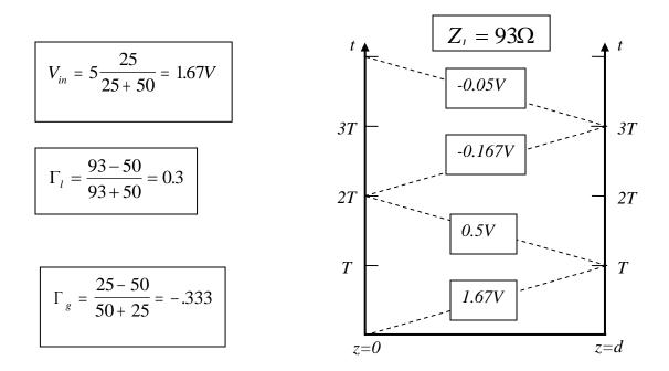
For the matched load  $Z_{in} = 50\Omega$ , the input and output pulses should both be 1.67V and be separated by the delay time, which they are. At the intermediate point (between the two lines), we see the signal at the source end appearing 1.8us later and the signal at the load end 1us later.
