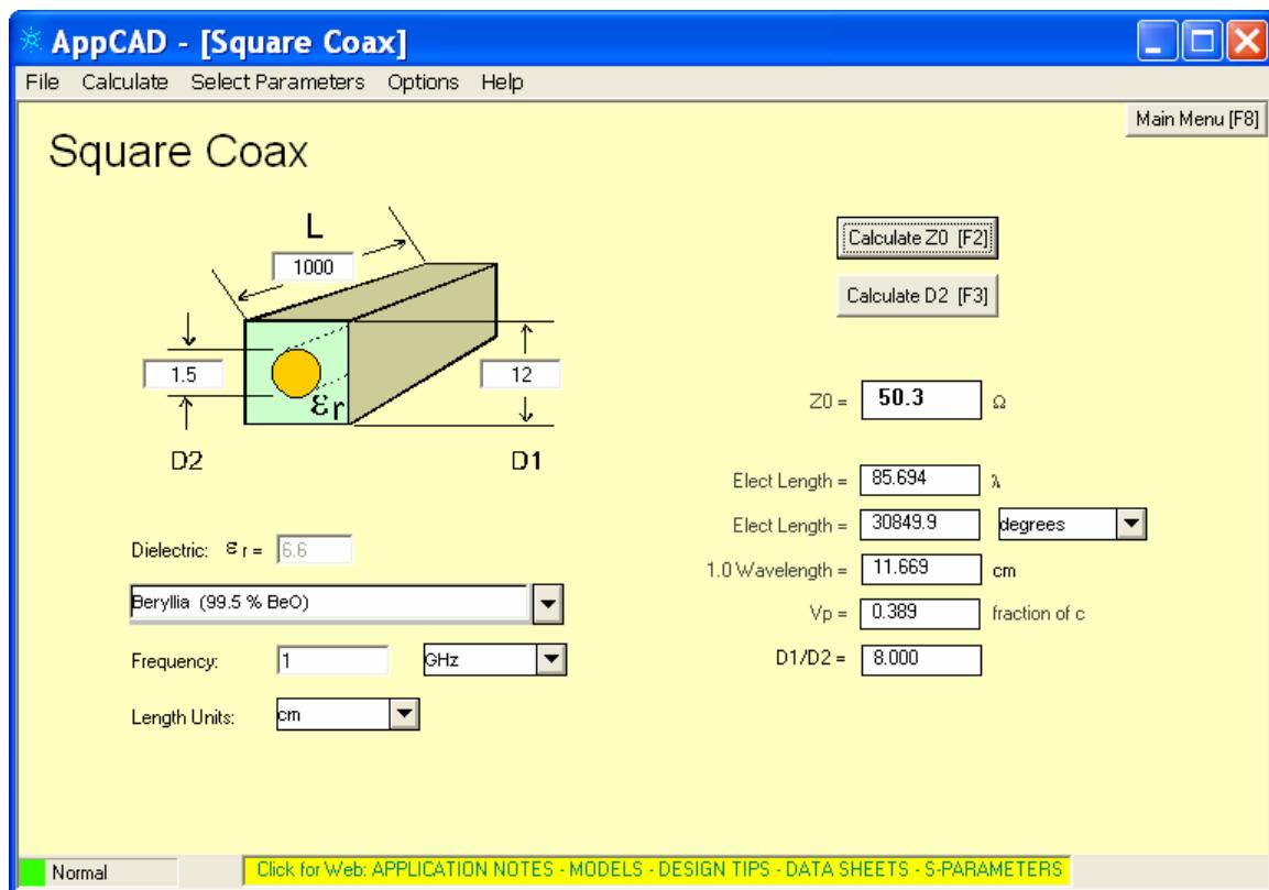
*From the options available, beryllia gives the best result. With a wave propagation speed of .389 the speed of light, we can figure out the capacitance and inductance per unit length.  $Z_o = \sqrt{\frac{l}{c}}$ ,  $v = \frac{1}{\sqrt{lc}}$ , so that  $c = \frac{1}{Z_o v} = \frac{1}{(50.3)(.389)(3e8)} = 170 \text{ pF/m}$ .*
