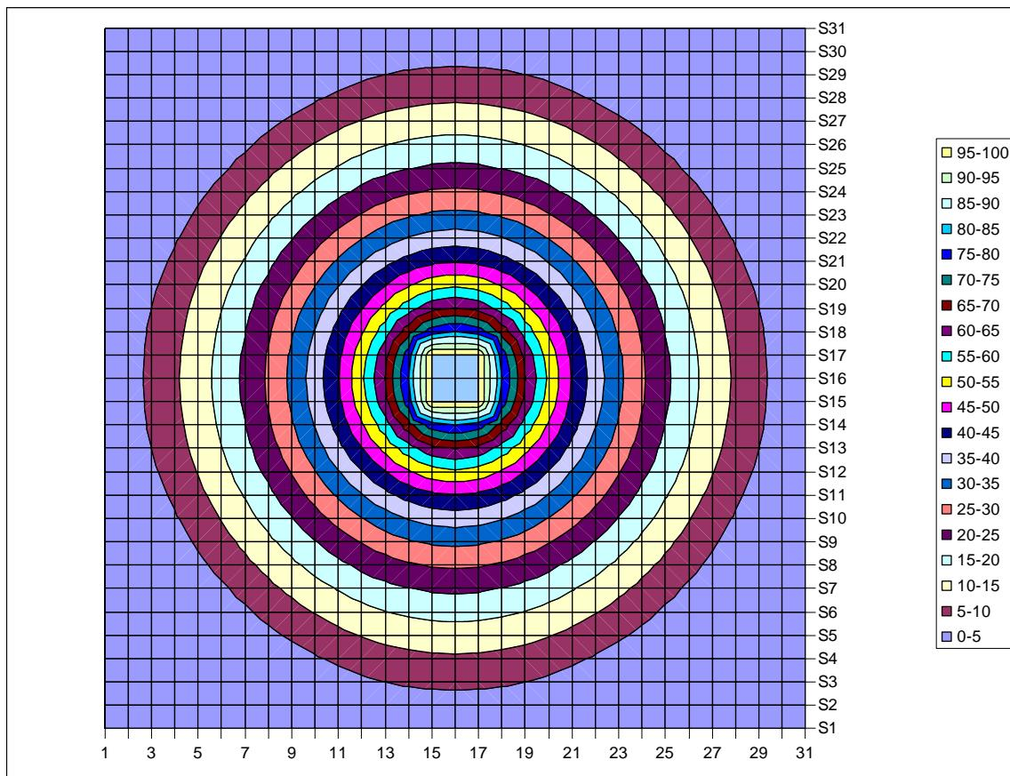
For the square outer conductor, the solution is similar to a problem done in the lecture slides. For the specific case considered, we have the following, shown sideways on the next page. The inner and outer capacitance values are not in agreement and, again, both are smaller than found with AppCAD.
