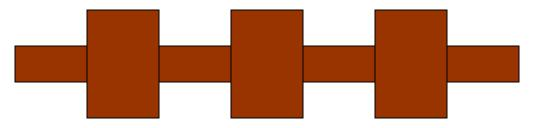
The width of the narrow regions is *3mm* while the wider regions are *9mm* in width. Each region is *6mm* long, so the total length of the resistor is *42mm*. Note, these are not really typical dimensions.
