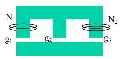
$$R_{1} = \frac{g_{1}}{\mu_{0}S} \quad R_{2} = \frac{g_{2}}{\mu_{0}S} \quad R_{3} = \frac{g_{3}}{\mu_{0}S}$$
