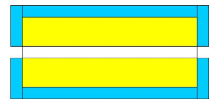
In the figure, the blue regions are iron and the yellow region is the coil. To make the analysis simpler, we will assume that the wires are wound only in a single layer so that we do not need to address their thickness. The simplified diagram is on the next page.
