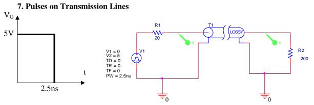
The 5V pulse is launched on the 20 cm long transmission line shown. For this line, the capacitance per unit length is  $1.7 \times 10^{-10}$  F/m and the inductance per unit length is  $1.1 \times 10^{-6}$  H/m. The propagation speed on this line was designed to be quite slow.
