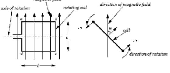
side view end view The coil has a height h and a length l and turns at a frequency  $\omega$ .
