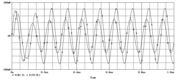
where the smaller voltage is the output signal. Disregard the variations at the beginning, since the signal does not reach steady-state until about 0.2us. Assume that we decide to use two sections of the lumped line to represent an 8 meter cable. We have a circuit that looks like
