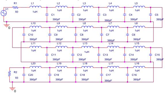
The physical circuit has one BNC connector at the input end and a BNC connector and two banana plug connector posts at the output end. This circuit can be modeled using PSpice to determine its frequency response. The input voltage as a function of frequency looks like:
