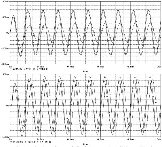
However, the input signals are the most similar for the second and third cases. This is probably due to the inadequacies of a lumped transmission line model with only two
