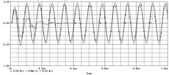
When using the lumped line, most groups found that the frequency for blocking was a bit lower than the ideal model would predict. Let us try such a lower frequency.
