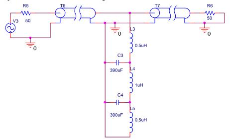
Notice that the short circuit now does not eliminate any of the components.
