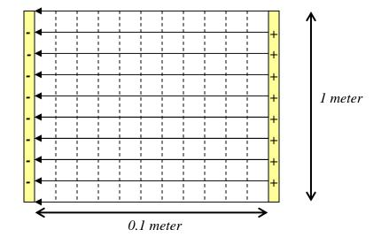
a. What is the capacitance of this parallel plate structure?
