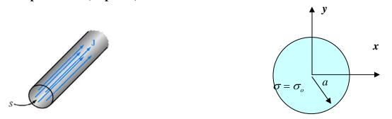
A long, straight, solid cylindrical conductor with a radius of a is shown above. The surrounding medium is free space. There is a total current  $I_o$  carried by this conductor directed **into the page**.
