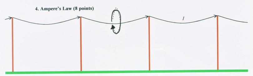
For an early telegraph line, the current in the line *I* is carried to the right in the wire and returns through the ground. If one applies Ampere's Law to the dashed loop surrounding the telegraph wire, which of the following describes the integral of the
