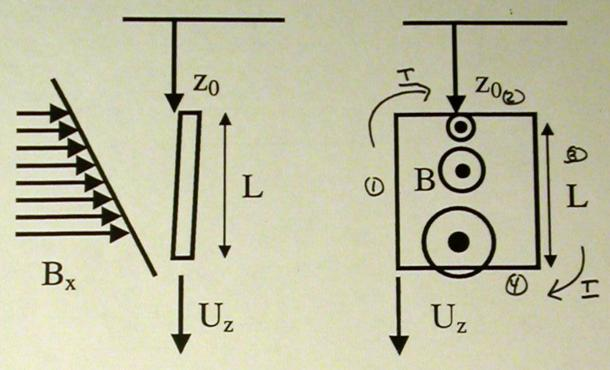
a) Find the flux linking the coil when the top conductor is at location  $z_0$ .
