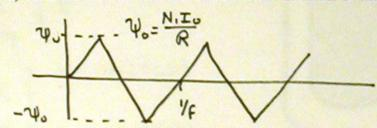
b) Find the flux linkage of each coil as a function of time. Sketch it
