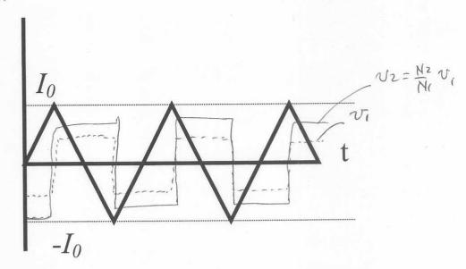
Sketch the voltage on winding 1 and the induced voltage on winding 2.
