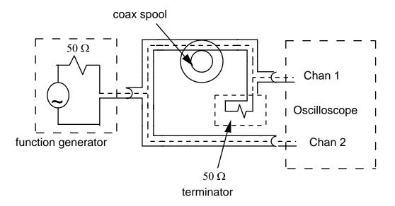
d. Measure the resistance of the center and outer conductors of the long coaxial cable. Do the same for the short cable. *Hint: remember to first measure the resistance of the cable you are using to connect to the multi-meter by short circuiting the two mini-grabber connectors together and then subtract this resistance from the resistance of the cables. Because you have to eliminate the effect of the measuring cable, your answer for the short cable may not be very accurate.*
