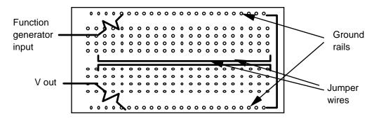
How large a voltage do you measure at  $V_{out}$ ? Is it what you expected? The two wires form a capacitor. Draw a circuit diagram with the capacitance of the wires unspecified. Be sure you include the internal impedance of the function generator. Vary the spacing between the wires and the frequency. What changes occur?
