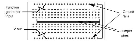
How large a voltage do you measure at  $V_{out}$ ? Is it what you expected? The two wires form a capacitor. Draw a circuit diagram with the capacitance of the wires unspecified. Be sure you include the internal impedance of the function generator. Vary the spacing between the wires and the frequency. What changes occur?
