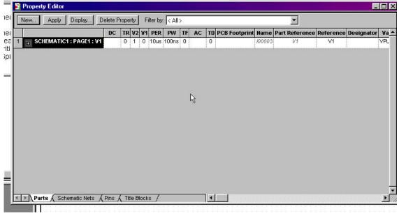
When you have finished, click on *Apply* and then close the window. Note that you should set the fall time, rise time and delay times to zero. Also, the AC and DC can be left blank. Next, double click on the transmission line and set its characteristic impedance to 50 and time delay to 400ns.
