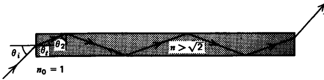
Figure 7-26 The index of refraction of a straight light pipe must be greater than \sqrt{2} for total internal reflections of incident light at any angle.
