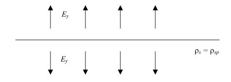
Step 3) The Gaussian surface is in the previous figures. The box has sides of length, *l*. Also, the box is symmetric about the surface charge distribution. We know that the field on a plane parallel to the surface charge is constant, so the <u>magnitude</u> of the field at some location y=C must be the same as that at the location y=-C. However, we do not know how the field behaves as a function of y.
