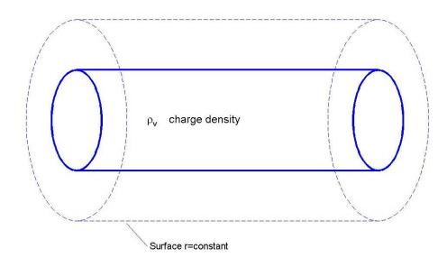
The field will point in the  $\hat{r}$  (or -  $\hat{r}$ ) direction for this geometry. For symmetry to apply, the charge density can only be a function of r.
