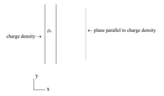
The field will point in the  $\hat{x}$  (or -  $\hat{x}$ ) direction for this geometry. For symmetry to apply, the charge density can only be a function of x.
