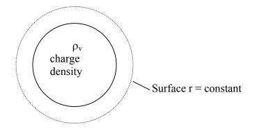
The field will point in the  $\hat{r}$  (or  $-\hat{r}$ ) direction for this geometry. For symmetry to apply, the charge density can only be a function of r.
