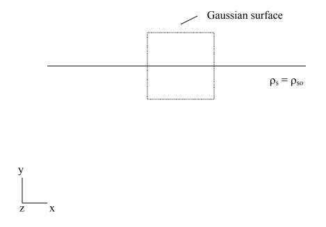
The Gaussian surface is drawn as an overhead view. In actuality, it has six sides:
