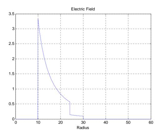
Before we can compare the actual values of the E fields, however, we must remember that the condition on this problem is that the voltage difference is the same, not the charge. In the plots above the charge is assumed to be the same.
