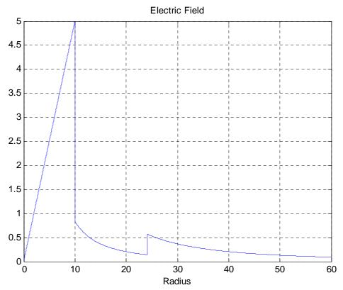
Note that the field increases linearly with radius out to *a*, then drops by a factor of 4 at the boundary with the plastic shell. At *b*, it increases by a factor of 4 and then decays toward zero.
