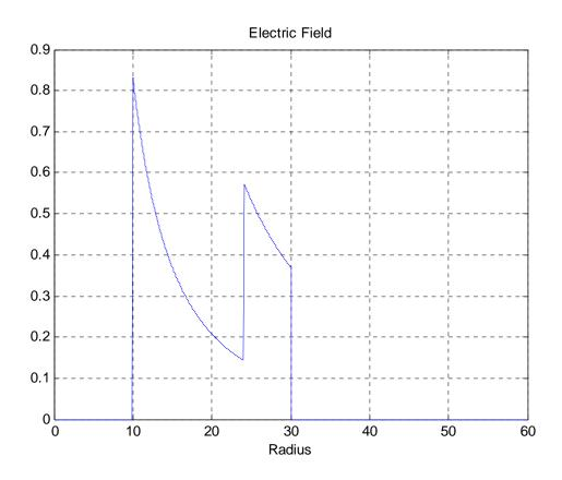
Finally, we reverse the location of the plastic shell, moving it to the outer region. We clearly see that the maximum E field is much larger in this case.
