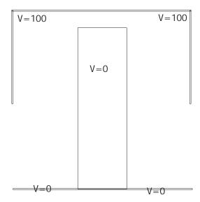
Extra Credit – Fill the upper half of the open region with Teflon. That is, everything from the bottom edge of the upper conductor to the top of the structure. Determine the capacitance for this more complex configuration and discuss the accuracy of your answer.
