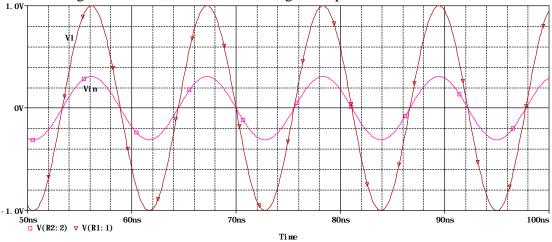
d. Finally, assume that four television sets are connected in series (people do very strange things, but probably not this) so that the load impedance is 300 ohms. Determine the reflection coefficient at the load  $\Gamma_L$  and sketch the standing wave pattern for this case. The input and output voltages for this case are:
