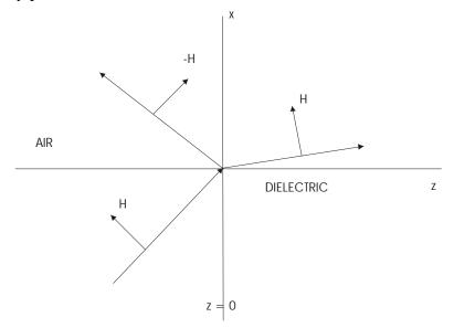
Now assume that **E** is replaced by **H**, as shown above. Note that the reflected **H** field is labeled  $-\mathbf{H}$  so that the same diagram can be used. By convention, we usually assume that **H** changes direction upon reflection. On the plot above, indicate the incident, reflected and transmitted angles:  $\theta_{I}$ ,  $\theta_{R}$ ,  $\theta_{t}$
