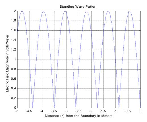
a. What is the wavelength  $\lambda$ , the wavenumber  $\beta$ , and the dielectric constant  $\varepsilon_r$  of the unknown material. What do you suppose Material X is?
