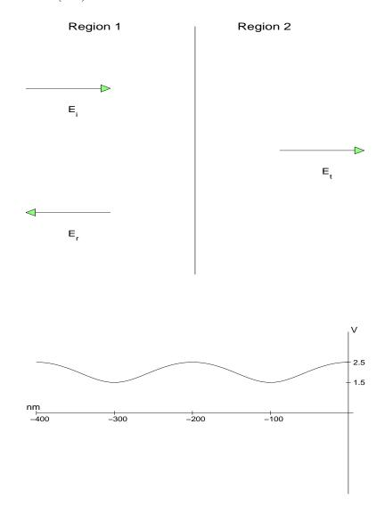
A plane wave is normally incident on a dielectric-air boundary. Both regions are lossless. The standing wave pattern is shown in the figure. (The pattern continues in the -x direction.)
