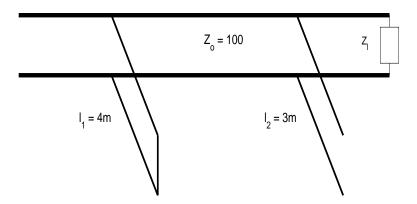
In the figure shown, two stubs are attached to the transmission line. Both the stubs and the line are lossless, have the same characteristic impedance, and have a velocity of 2E8 m/s. One stub is open and the other is short, as indicated on the figure. What frequency(s) will be blocked at the load? (15)
