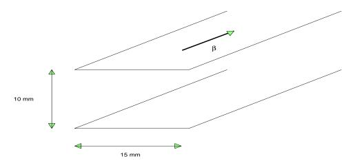
A parallel plate transmission line is shown in the figure, with the direction of propagation indicated by  $\beta$ . Draw a cross sectional view of the line and label the voltage, current, electric field lines and magnetic field lines at an arbitrary point. Only the forward propagating wave should be considered. All vector must have an associated direction. Indicate the direction of propagation in your figure (into the page or out of the page)(8)
