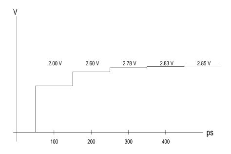
The voltage at the load of a short transmission line is shown in the figure. The line has a velocity of 100E6 m/s and the source is DC and switches to 5 V at t = 0. If the load impedance is 100  $\Omega$ , what is the source impedance? (5)
