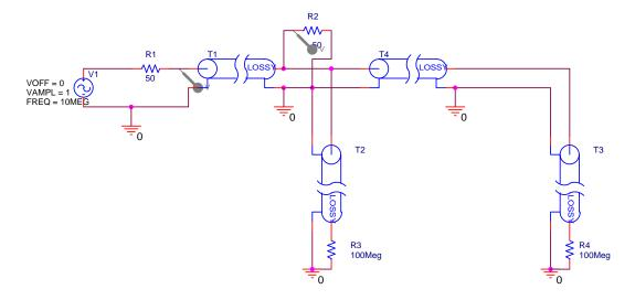
You should use double or triple stub circuits to build your filter for this project. You can locate double stubs directly across the load instead of between the load and the source.
