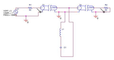
At the resonant frequency of the LC combination, there will be a short across the line and the input signal will not reach the load. Both of these can work, but there are other options that generally work better, including the more elaborate discrete component filters in the <u>www.dxing.com</u> link. Several options follow.
