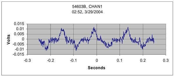
The signal is noisy because the coil does not make good contact at all times. It is not a good sine wave since the B field is not constant. From this signal, you can tell the frequency of rotation and the maximum induced voltage. Use this information to justify your estimate of the contribution from the back EMF in your motor design. You can also use this information to get a rough idea of the average B field, if you also know that this coil had about 7 turns of wire.
