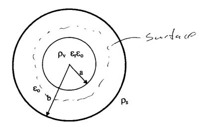
The above figure represents two spherical charge distributions, a volume charge for the region r < a and a surface charge located at r = b, where a < b. The total charges of each distribution are equal and opposite. The volume charge is distributed throughout a dielectric material with permittivity,  $\varepsilon_r \varepsilon_o$ , The rest of the domain is free space.
