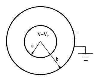
A cylindrical capacitor is shown above. A dielectric material,  $\varepsilon_r = 4$ , fills the space between the conductor. The voltage on the inner conductor is Vo and the outer conductor is grounded. The dimensions are shown.
