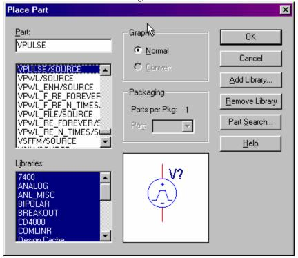
Click on the OK button. You can then place the symbol for the source anywhere on the schematic window. The other parts we will need are R for two resistors and T for transmission line. Once you have selected and placed these parts, your window should look something like the following:
