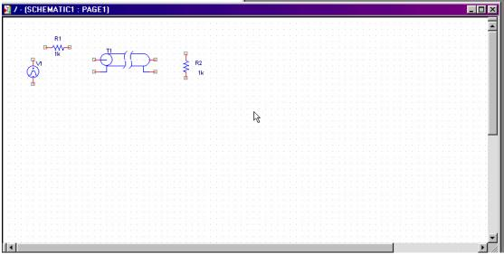
When you first place the resistors, you should see that they are positioned horizontally. To rotate the load resistor at the right, click on it and then hit the *R* key in your computer keyboard. You can also choose *Edit*, *Rotate* to accomplish the same thing.
