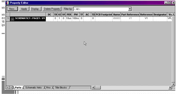
When you have finished, click on *Apply* and then close the window. Note that you should set the fall time, rise time and delay times to zero. Also, the AC and DC can be left blank. Next, double click on the transmission line and set its characteristic impedance to 50 and time delay to 400ns.
