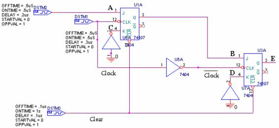
a) The following figure shows the clear signal, the clocks and the input at A. Draw the traces at B, C, D and E.
