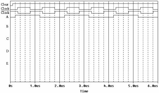
b) If the clock for a counter (74393) was attached to signal A, what would the output look like after 3.0us. (Assume the counter has also been cleared, therefore QA=0V, QB=0V, QC=0V, QD=0V at time 0s). Express your answer in volts.
