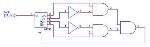
ii. Write down the complete counting cycle of the counter (in decimal), in the above formation. Show that the counter resets after the counting cycle has finished. (3 pts)
