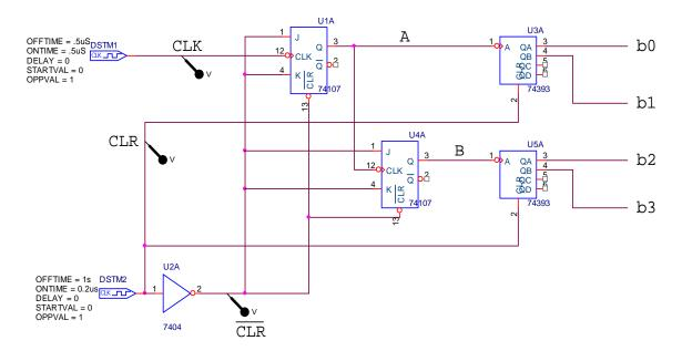
a) In the above circuit, the CLR signal resets the counters at t=0.2us and the ~(CLR) resets the flip flops at t=0.2us. The input clock to the first flip flop (UA1) is the CLK signal. These signals are shown below. Draw a trace for the signals at point A and point B. Also draw a trace for the output signals: b0, b1, b2 and b3. Note that the flip flops and the counters all trigger on the falling edge of their input clocks. (2 points per trace=12 points)
