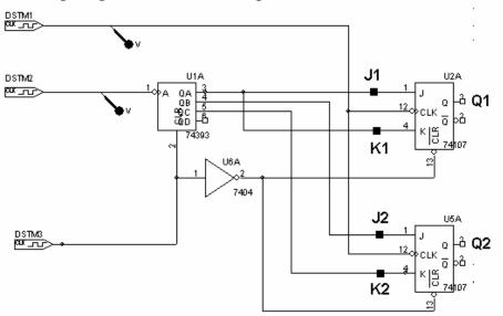
a) Complete the timing diagram for the circuit above. Note that the first trace shown is DSTM1 (flip flop clock), the second trace shown is DSTM2 (counter clock), and DSTM3 provides an initial reset pulse to both of the devices. You can assume that all outputs are initially 0 and that all three devices change on the falling edge of the clock. Draw traces for all six of the points indicated: (J1, K1, Q1, J2, K2, Q2)
