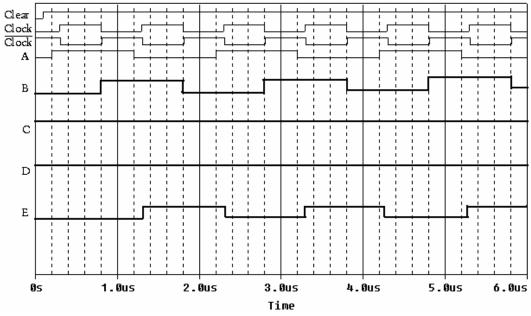
[Some explanation: C and D are inverted from ground. This means they are always high. Note that the flip flops only change on the falling edges of the clock. The first flip flop will look at J and K when Clock goes down at 0.8 us. Since at that time A(=J) is high and C(=K) is high, the flip flop toggles and B goes high. The next time that Clock goes high to low at 1.8us, A is low and C is still high. This time, the flip flop should be equal
