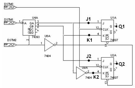
a) Complete the timing diagram for the circuit above. Note that the second trace shown is DSTM1 (counter clock), the first trace shown is DSTM3 (flip flop clock), and DSTM2 provides an initial reset pulse to both of the devices. You can assume that all outputs are initially 0. Draw traces for all six of the points indicated: (J1, K1, Q1, J2, K2, Q2) (*3 points each* = 18 points)
