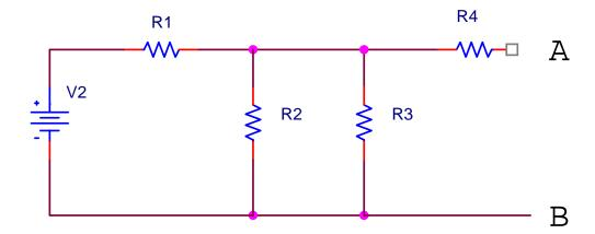
Let V2=12V, R1=50 ohms, R2=1K ohms, R3=2K ohms, and R4=500 ohms.
