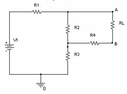
Let V1=12V, R1=50 ohms, R2=10K ohms, R3=2K ohms, and R4=500 ohms. RL represents the load placed on the circuit between points Aand B.
