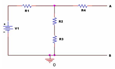
In the circuit above, V1=6 volts. R1=  $50\Omega$ , R2=  $500\Omega$ , R3=  $800\Omega$ , R4=  $3000\Omega$
