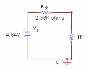
d) (4 points) Find the voltage between A and B for this circuit with a load of 1K ohms.
