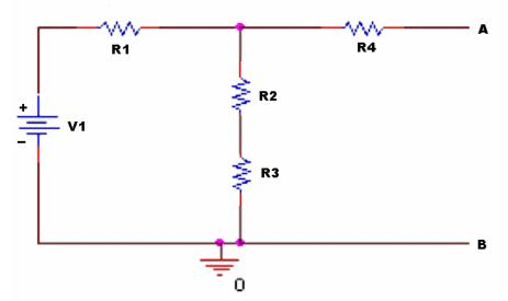
**A:** In the circuit above, V1=6 volts. R1=  $50\Omega$ , R2=  $500\Omega$ , R3=  $800\Omega$ , R4=  $3000\Omega$
