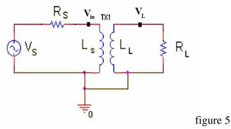
When  $R_S$  is large, we need to use  $V_{in}$  to find the voltage relationship instead of  $V_S$ . In this case we can use  $Z_{in}$  directly.
