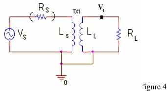
When  $R_S$  is small, we can use the source voltage as the voltage in the relationship. First we use the loop equations for the two circuits.
