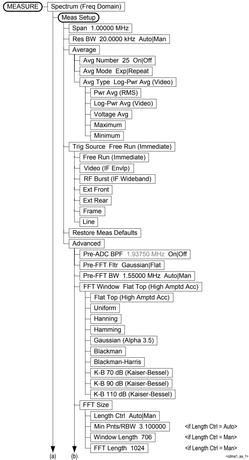
Figure 6-9 Spectrum (Freq Domain) Measurement Key Flow (1 of 3)
