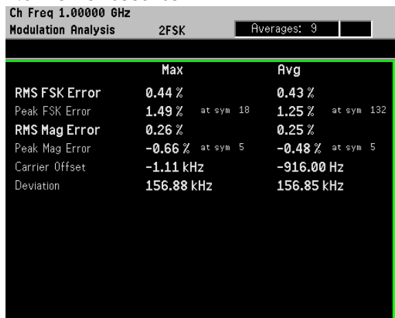
Figure 2-55 FSK Numeric Results
