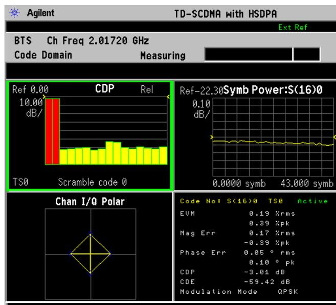
**Step 13.** Press Trace/View, Demod Bits to display a combination view of the code domain power, symbol power, and the I/Q demodulated bit stream data for the symbol
