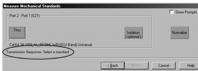
Figure 43. Response calibration and associated standard selection for Reflection Response and Transmission Response.
