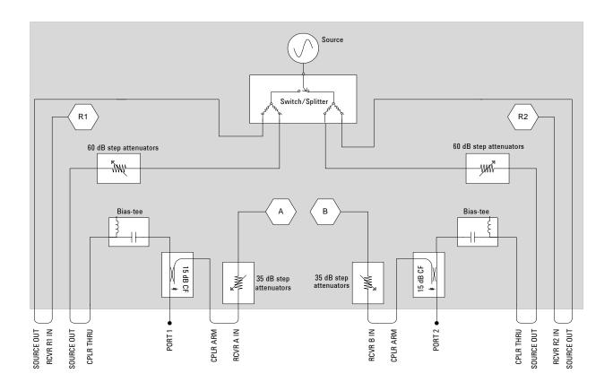
The above diagram is a block diagram of an Agilent E8362/3/4B MW PNA network analyzer with options 014 and UNL.
