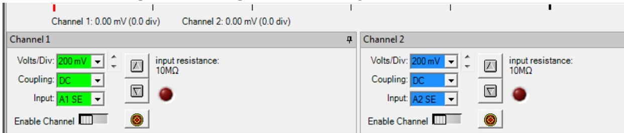
Again, we will see what these all mean by changing things to see what happens. However, we can notice one thing at this point. The input for channel one is A1+ (pin 1) and for channel 2 is A2+ (pin 4). A1 SE means the measurement is being made between A1+ and ground (GND) and A2 SE means the measurement is being made between A2+ and GND.
