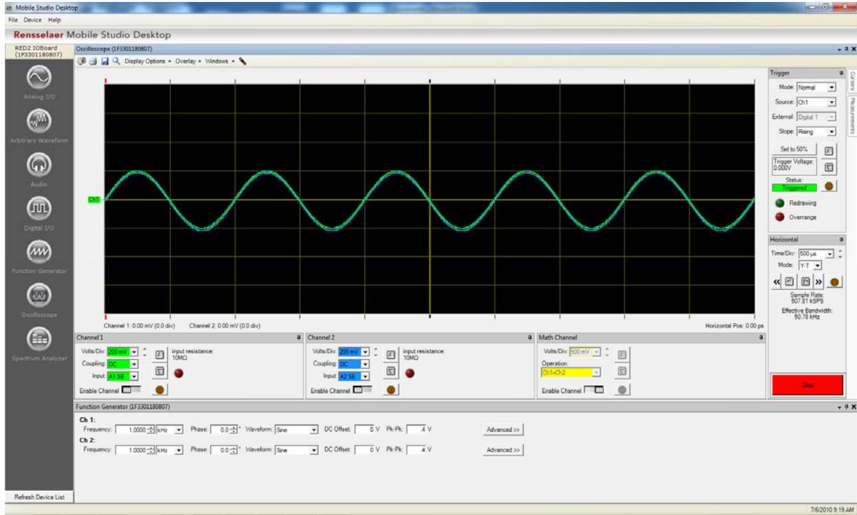
Because of calibration differences between boards, your two sine waves may be somewhat separated in the vertical direction. We will not worry about this phenomenon. For simplicity at this point, we will turn off channel 2 and only look at channel 1. Click on the 'Enable Channel' button under Channel 2 and the blue curve should disappear.
