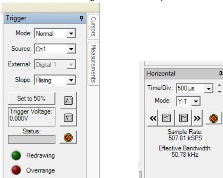
The trigger tells the oscilloscope when to start making the measurement. The horizontal sets the time during which the measurement is to be made.
