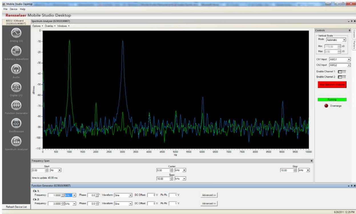
You should try some different frequencies, listen to the sounds and watch how the display changes on the spectrum analyzer. Do the changes you observe in the spectra make sense in terms of what you can hear and what you have set the function generators up to do?
