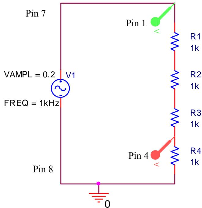
Describe what you observe. Does it make sense to you? Move the connection to pin 4 (channel 2) so that there are two resistors above and below it in the series combination. Again describe what you observe. Finally, move it up one more resistor so that there is only one resistor above it and three below (between it and ground). Describe what you observe.
