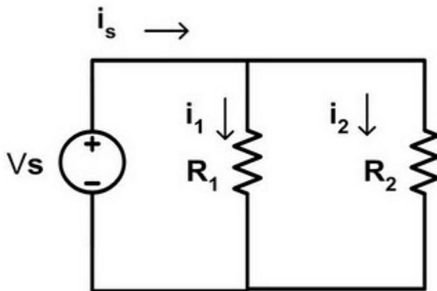
Here we will use  $R_1 = 1k\Omega$  and  $R_2 = 33k\Omega$ . From your calculations in the Resistors activity, determine the combined resistance  $R_T$  of the two resistors in parallel. Then, determine  $i_s = \frac{V_s}{R_T} = \frac{9V}{R_T}$ . Use Ohm's Law to find the other two currents and verify that  $i_s = i_1 + i_2$
