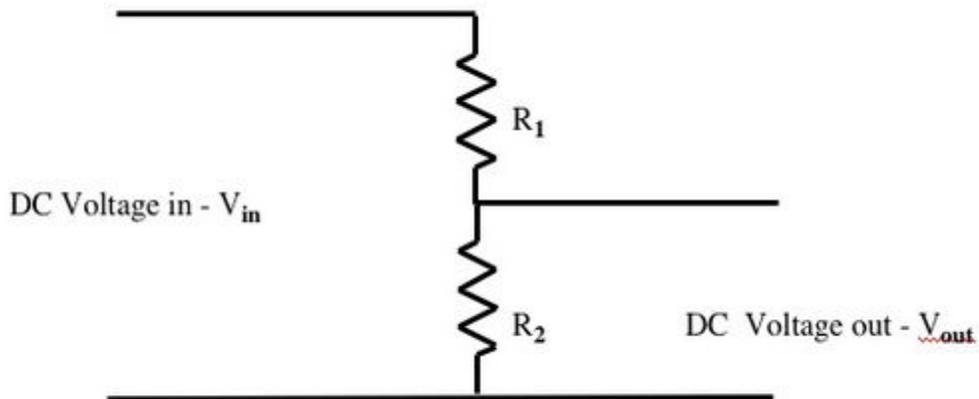
Set up this circuit using  $1\text{k}\Omega$  resistors for both  $R_1$  and  $R_2$ . From Ohm's Law analysis, based on the assumption that the current through both resistors must be the same, we know that
