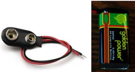
The wires used in the connector are stranded, so they are a little difficult to attach to the protoboard, but you will be able to do this with a bit of practice. However, it is best to leave them attached, and connect to resistors, etc. using the jumper wires provided.
