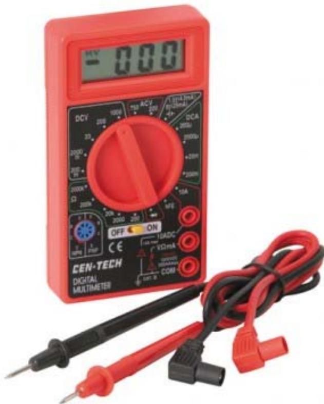
Note that there are three places to connect the probe wires. Plug the black lead at the bottom and the red lead in the middle. To use the meter, you must set the function with the dial. To measure resistance values you should turn it to one of the options in the area marked with the Greek letter  $\Omega$ , the symbol for Ohms, the unit of resistance. Select the range to be just larger than the value of your resistor (read from the colored stripes).
