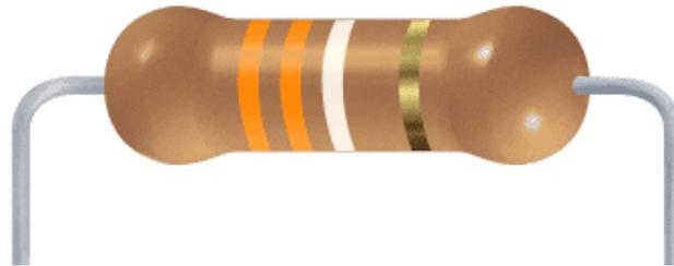
The colored stripes tell us what the value is of the resistor. Only the first three stripes are used for this purpose. The first two stripes are read like a regular number with each color representing a specific digit.
