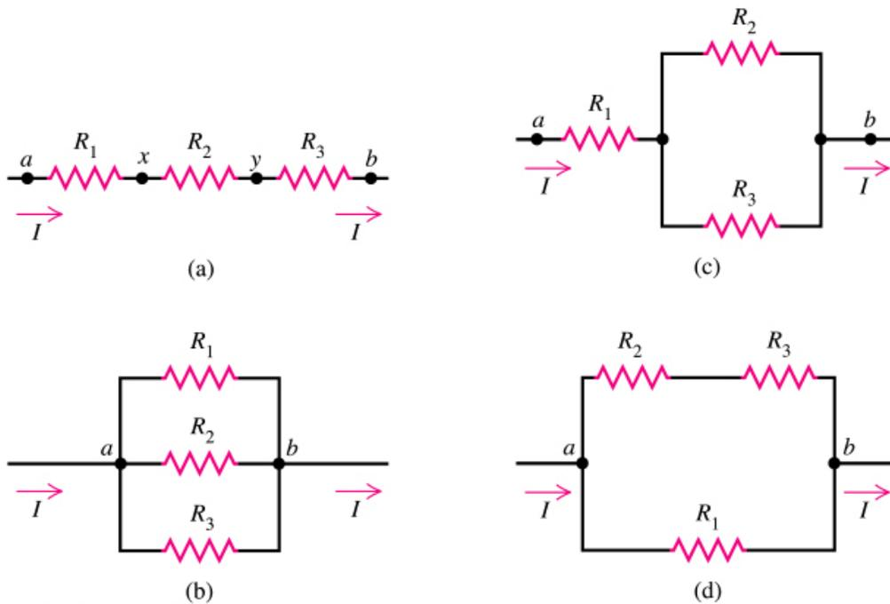
Two resistors in series: Combine a  $1\text{k}\Omega$  and a  $100\text{k}\Omega$  resistor in series on your protoboard. Calculate and measure the combined resistance.
