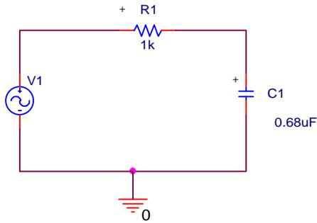
For the low-pass filter shown, the calculated frequency response is shown in the following plot.
