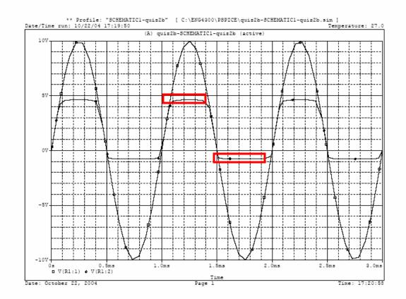
I am assuming that region 1 is the upper region which cuts off at about 4.7 volts and region 2 is the lower region which cuts off at about -0.7 volts.
