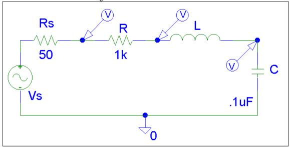
The following plot is obtained for the voltages at the indicated points in the circuit.
