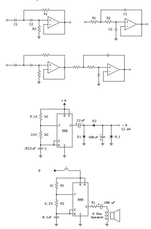
Shown above are five circuits. They are a band-pass filter, a tone generator, a low-pass filter, a +9v to -5v DC converter, and a high-pass filter. Identify which is which. Explain your answer.
