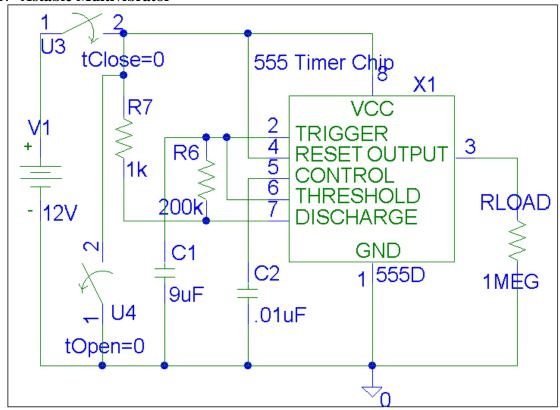
The circuit above has been simulated using PSpice. Using PROBE, the voltages at pins 2, 6, 7, and 3 have been displayed. Which of the three following plots will be observed? Since all four voltages are shown on the same plot, indicate which curve corresponds to which voltage. Explain your answer below.
