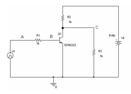
a) Redraw the circuit when the diode in the transistor is "off". Show the transistor as a switch in the appropriate position. What is the value of the voltage at point C? (6 points)
